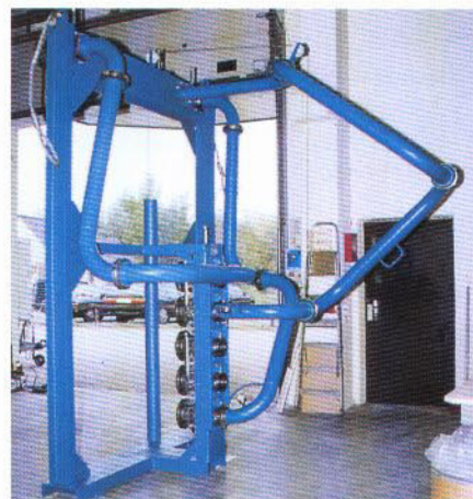
Swivel arms on the manual matrix manifold with sliding couplings in the swivel joint and connection
