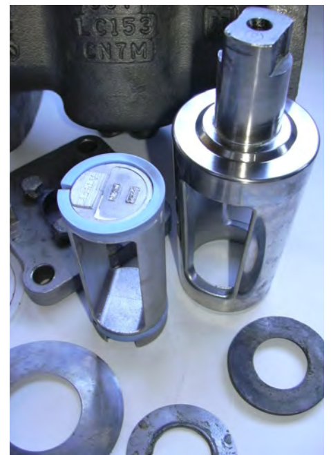
Disassembled KLINGER valve following 1 year of testing
