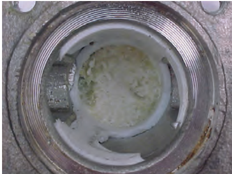
Competitor's valve, port without lips
