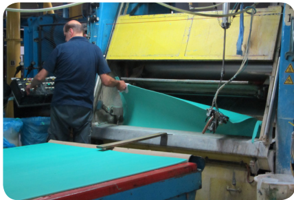
A sealing sheet is removed from the calender
