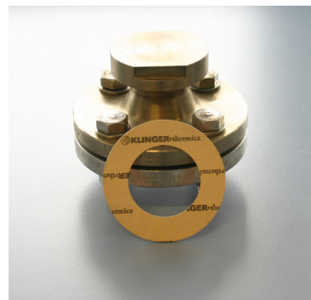
A seal in front of a test flange for determination of the chemical resistance
