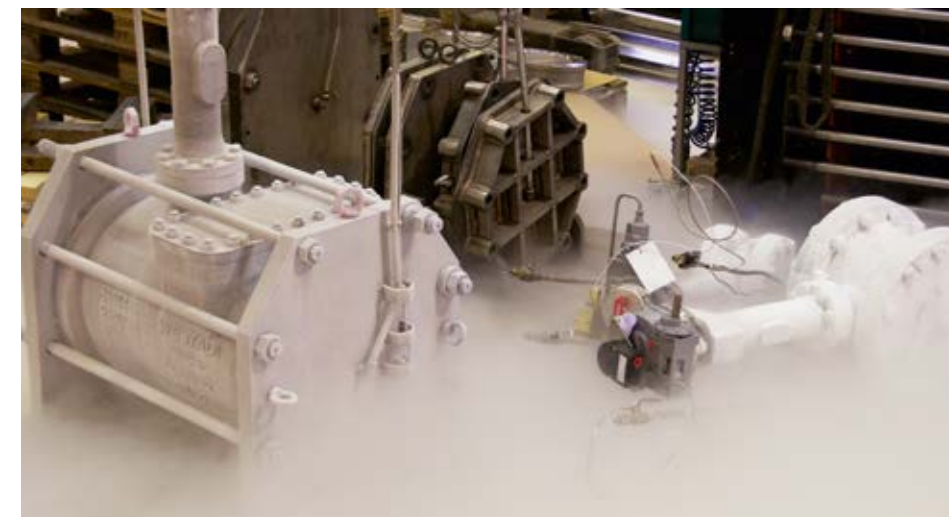
A cryogenic butterfly valve undergoes testing at -192^\circ\text{C}
