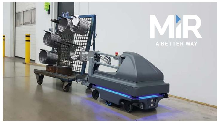
On the road again: MiR covers a distance of more than 10 kilometers on a daily basis. The robot reliably brings components wherever they are needed
